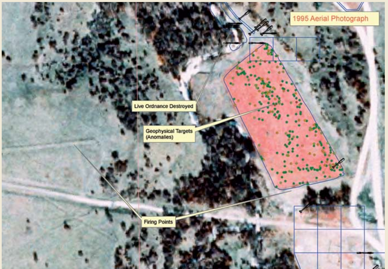
highest potential of ordnance. The firing points indicate the point from where the ordnance was fired. All live ordnance destroyed indications refer to those destroyed during the current project. Field data are entered using PDAs and fed into a database that is directly linked to the GIS.
